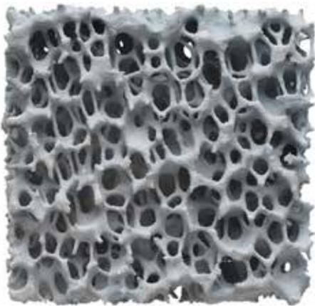
Optiflo SF: Silicon carbide ceramic foam filter
