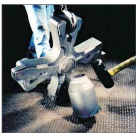
Abrasive wheel cutting is eliminated when using silica mesh for a breaker material.
