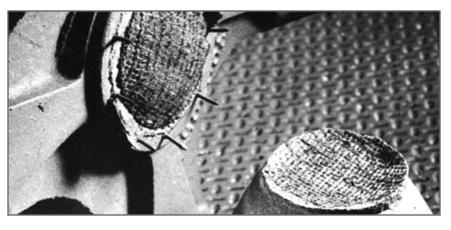
Silica mesh can be used for riser knock-off as a riser removal plane
